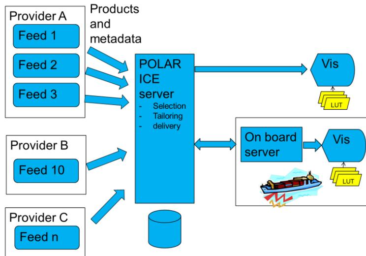
Figure 2. The POLAR ICE System – sea-ice products from several providers are made available to a central server where a Catalogue of available products, is produced. The Visualisation system enables the users to order the products in a tailored format. It is possible to change the colouring scheme at the end user’s side and this is applied to products representing the same physical ice parameter.
