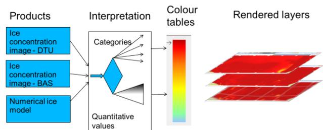
Figure 1. Schematic drawing of rendering process. The source products are interpreted using predefined rules, then the categories and the physical values are coloured according to parameter specific colour tables.
