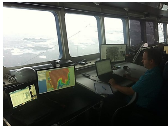
Figure 6. POLAR ICE running on the Finnish icebreaker Otso’s bridge off the coast of Greenland.
