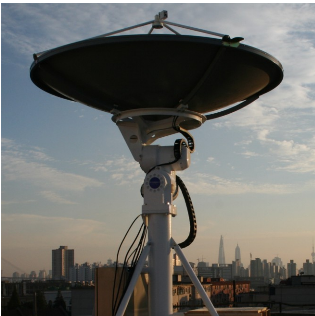
VxEos 2.4m X-band only antenna during installation at Shanghai Ocean University, China in 2007.
